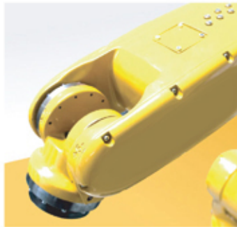
Electrical and pneumatic near tool flange.
