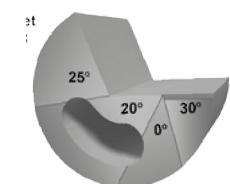
Facet grinds are preferred on specific applications, or when regrind fixtures limit the cam type sharpenings. They can be ground to various slash type angles with good performance and allow a greater amount of clearance for coolant to cool the chip at the cutting edge. This grind is standard on most European applications.
