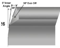
For applications requiring drilling flat bottoms. It can also be ground for a completely flat bottom, or on difficult materials; use to qualify bottoms only.
