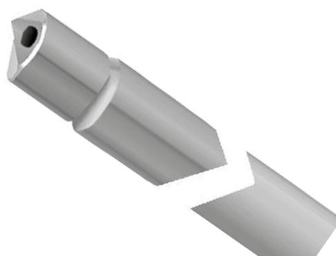
Step drills have manufacturing limitations depending on extreme diameter ranges in the steps. Special carbide developing may sometimes be necessary due to the coolant hole location. Additionally chip breakers may be required due to the lack of an inside angle which curls and breaks the chips under normal circumstances. Ideally using this type of drill yields virtually no eccentricity between diameters.
