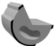
For use in aluminum and brass for best hole finish and for intersecting holes and interrupted cuts, or extra O.D. support and burnishing. Use with wood and plastic in combination with .0015/.002" back taper. Do not use in high nickel content materials due to high burnishing forces (micable).
