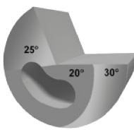
General purpose stock drill grind for steel, inconel and stainless steel, most often used with stock 'R1' O.D. contour.
