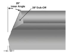
In aluminum and brass, use this grind with 'R4' O.D. contour for best hole finish.
