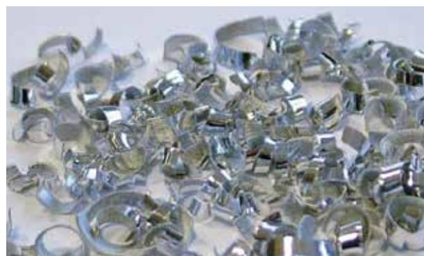
**With 3D-chip breaker: Breakage chips**
