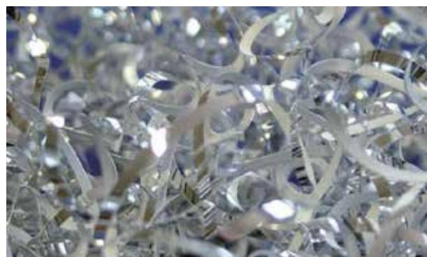
**Without 3D-chip breaker: Flow chips**
