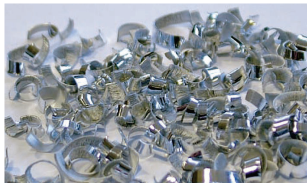
With 3D-chip breaker: Breakage chips
