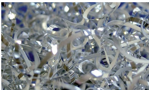
Without 3D-chip breaker: Flow chips
