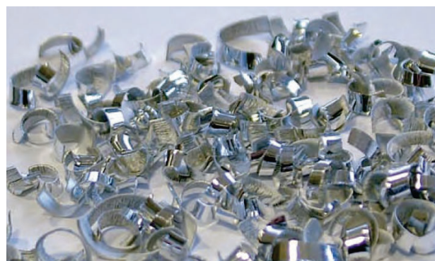
With 3D-chip breaker: Breakage chips
